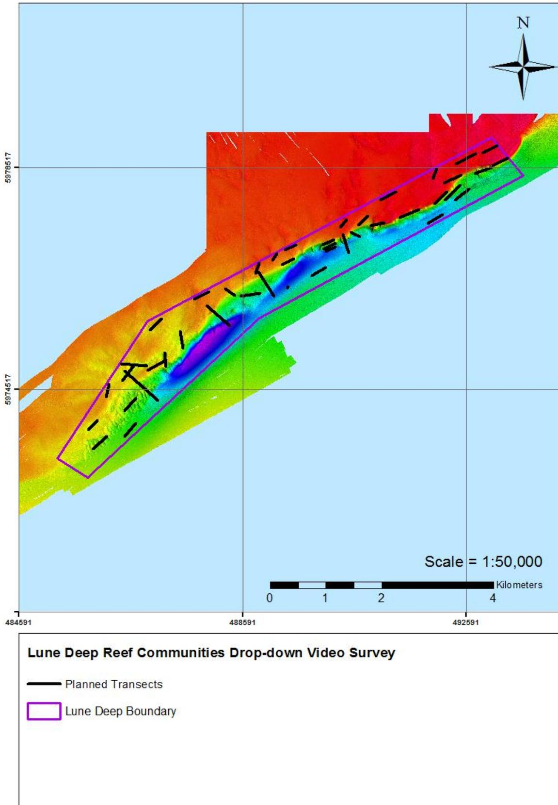
**Figure 2.1:** Location of planned camera transects for the 2015 Lune Deep drop-down video survey overlying multibeam bathymetry data supplied by Natural England
