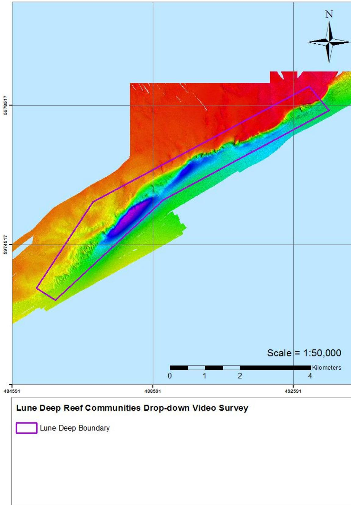
**Figure 1.3:** Multibeam bathymetry acquired by the Maritime and Coastguard Agency in 2008 and 2009 in and around the Lune Deep
