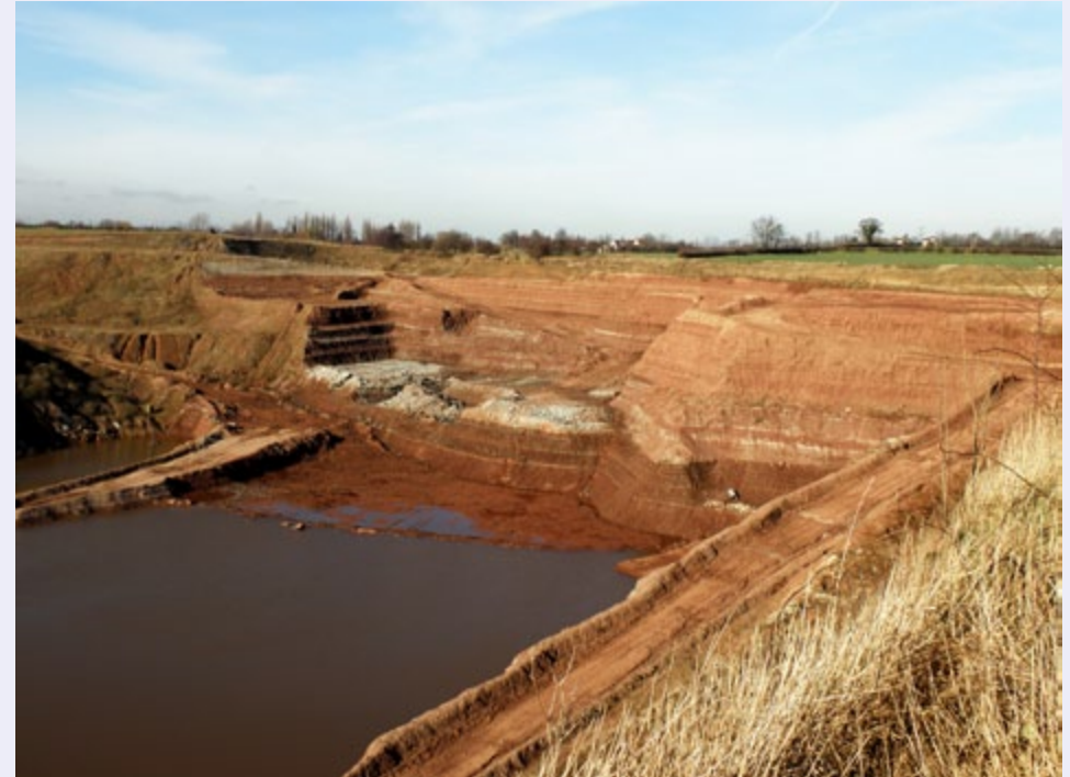
Ibstock brick pit, just one of a number of pits exploiting the extensive deposits of clay for the manufacture of bricks and tiles.
