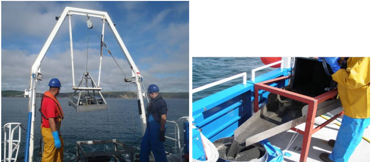
Figure 5. Mini-Hamon Grab (left), and equipment for sieving benthic fauna samples (right)
