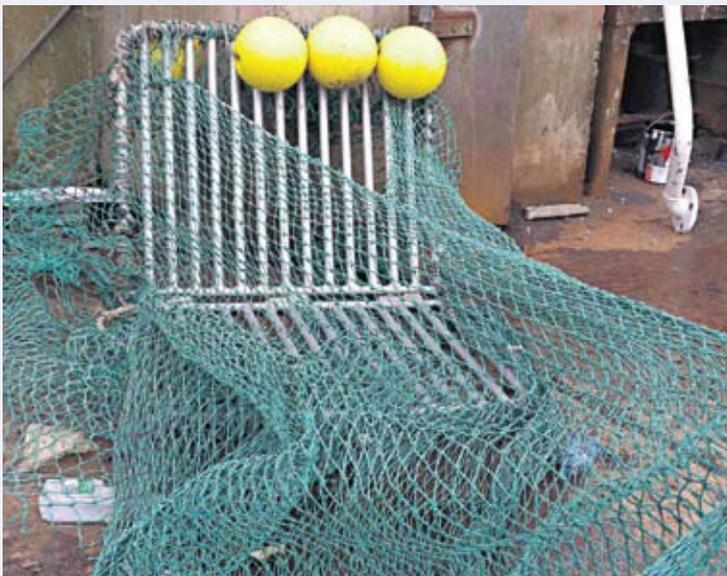
A 'Swedish grid'. This separator panel can be inserted into a *Nephrops* trawl to minimise bycatch of fish
