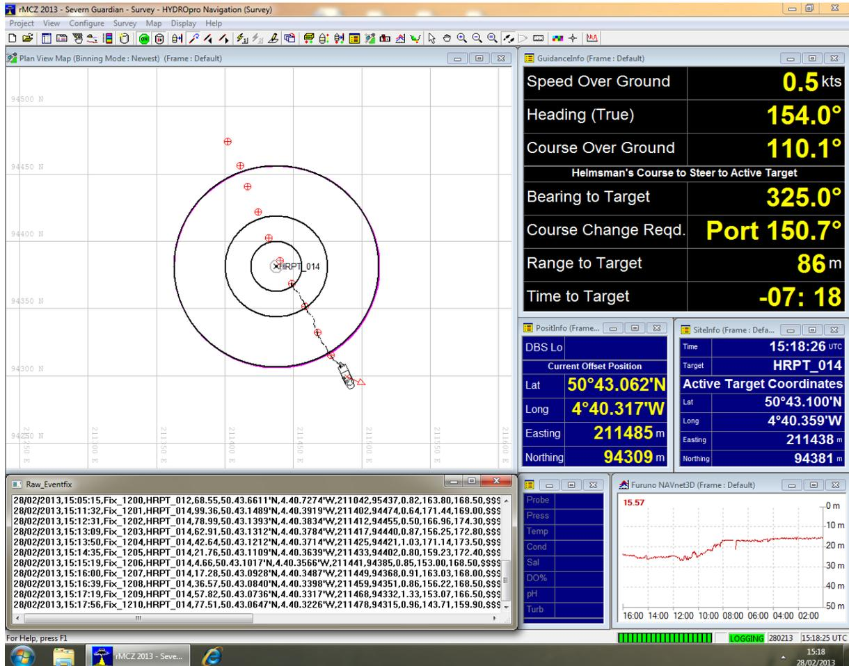
Trimble® HYDRO<sup>pro</sup>™ software screen grab displaying real-time navigation and survey data acquisition.
