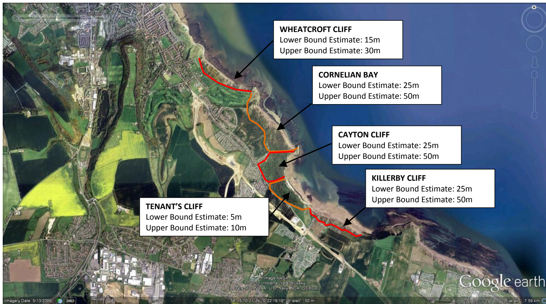
Figure 3 Cayton, Cornelian and South Bays SSSI: predicted 50-year recession rates of site boundaries (Image source: Google Earth). The coloured lines show the approximate cliff unit boundaries.
