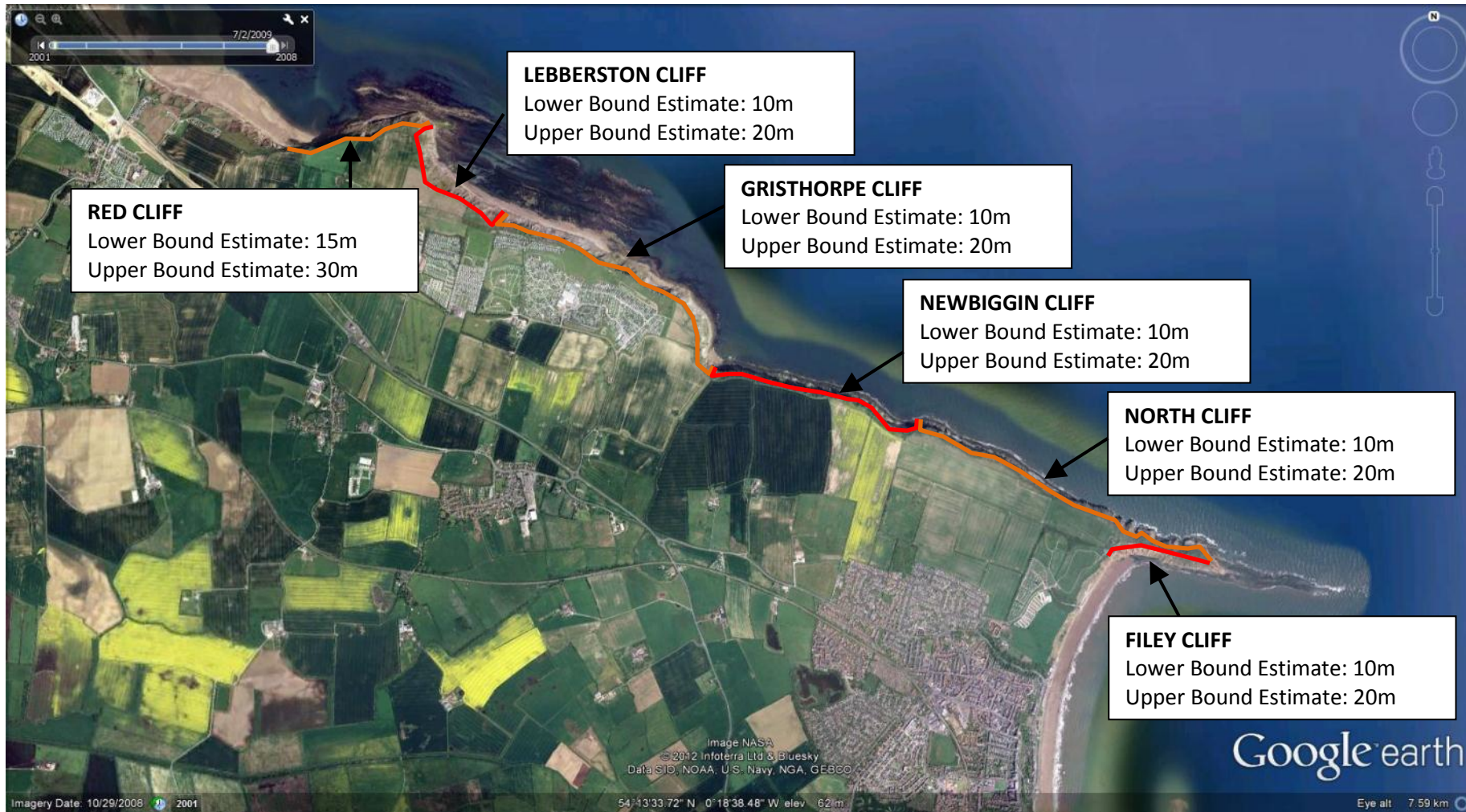
Figure 4 Filey Brigg SSSI, Gristhorpe and Redcliff SSSI and the proposed extension between Filey Brigg and Gristhorpe Bay: predicted 50-year recession rates of site boundaries (Image source: Google Earth). The coloured lines show the approximate cliff unit boundaries.
