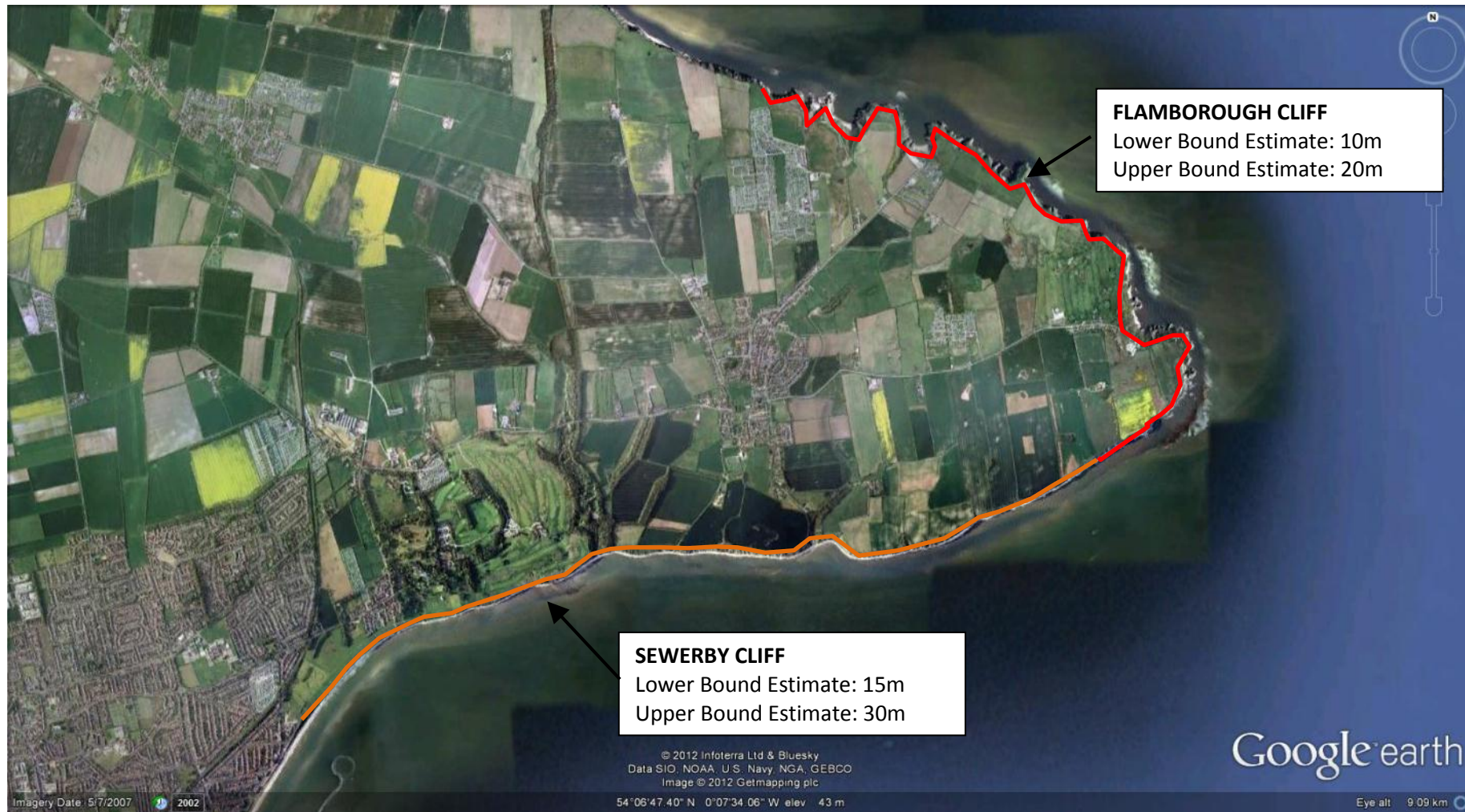
Figure 6 Flamborough Head SSSI (Long Ness to Sewerby): predicted 50-year recession rates of site boundaries (Image source: Google Earth). The coloured lines show the approximate cliff unit boundaries.
