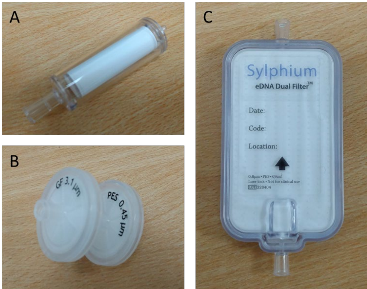
Figure 5. Filter types. Images of each different filter type used: A) 0.22µm Sterivex PES filter; B) 0.48µm PES filter in combination with 3.1µm glass fibre pre-filter; C) 0.8µm Sylphium PES filter (© Helen Rees, ADAS).
