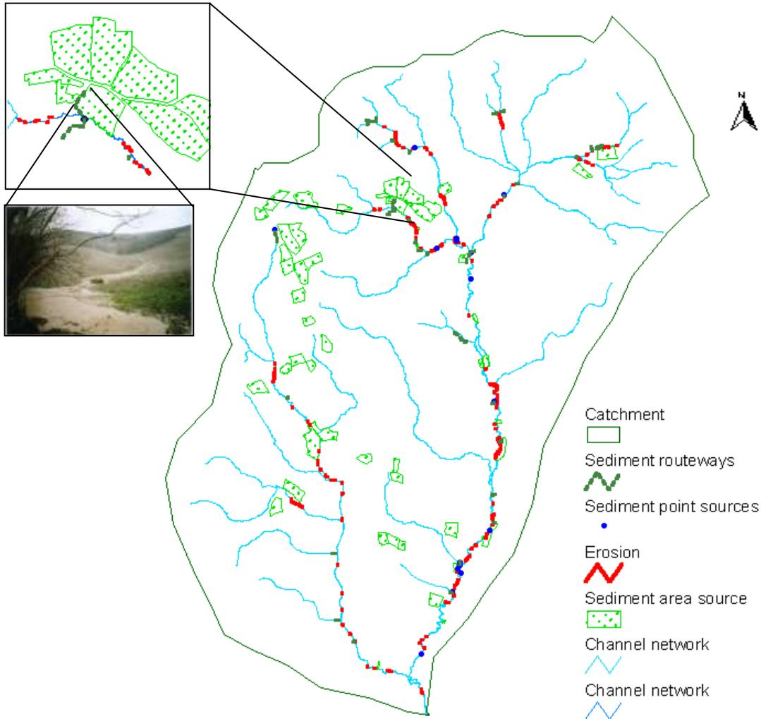
**Figure G** Example fluvial audit of sediment sources and routeways identified by field reconnaissance and air photo interpretation. (Ground-truthing during storm events and by stakeholder interviews provide higher levels of confidence)
