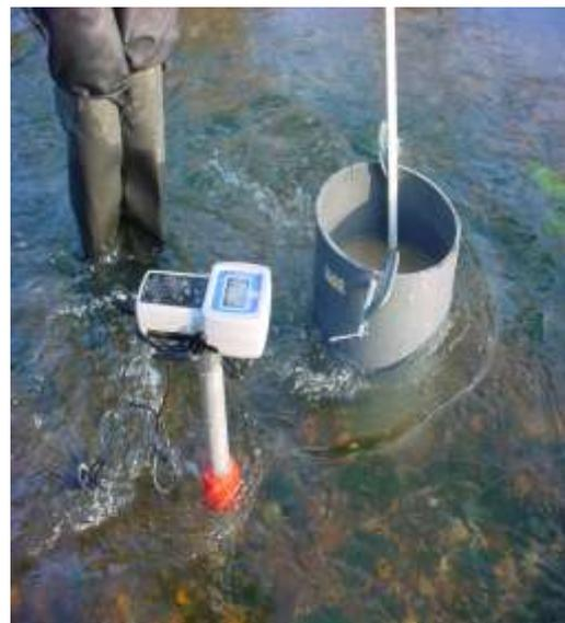
**Plate 1** Use of bed material disturbance within a stilling well - River Nar, Norfolk: location on spawning riffle (left) and detail of dissolved oxygen meter (right)
