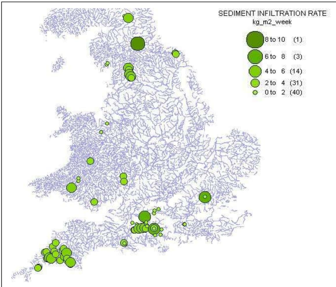
**Figure A** Fine sediment infiltration rates in UK rivers
