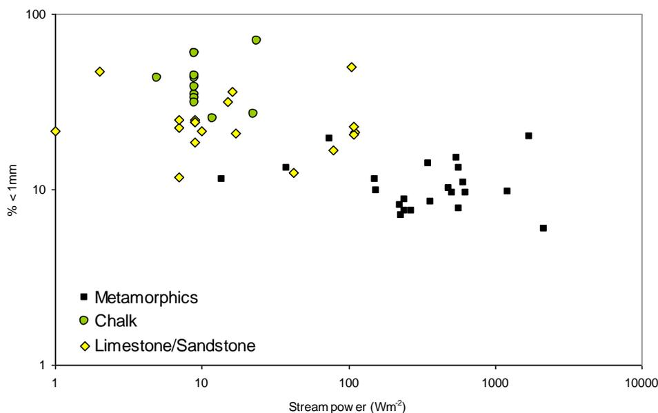
**Figure B** Relationship between stream power and the level of fine sediments recorded in freeze core bulk gravel samples (after Milan and others 2000)
