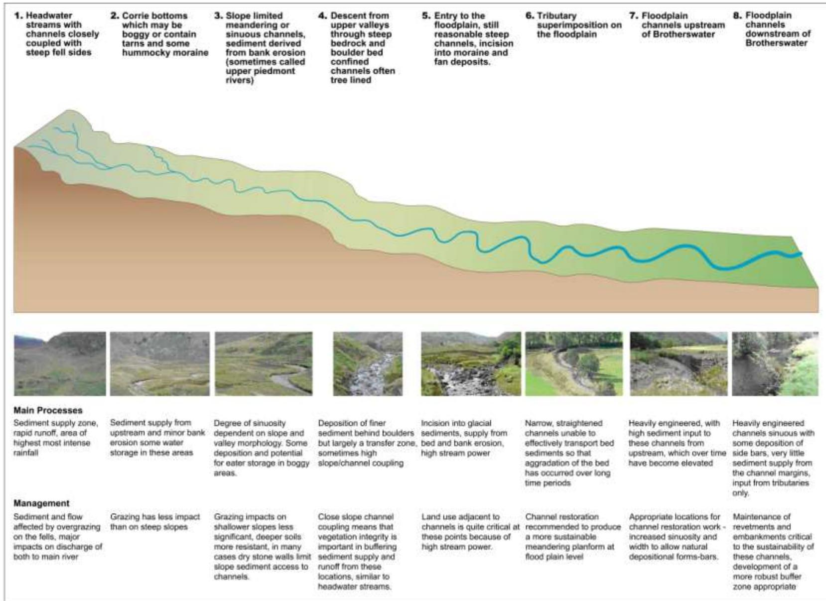
Figure F A typology of the upland sediment delivery system: Goldrill Beck (source Orr 2003a)
