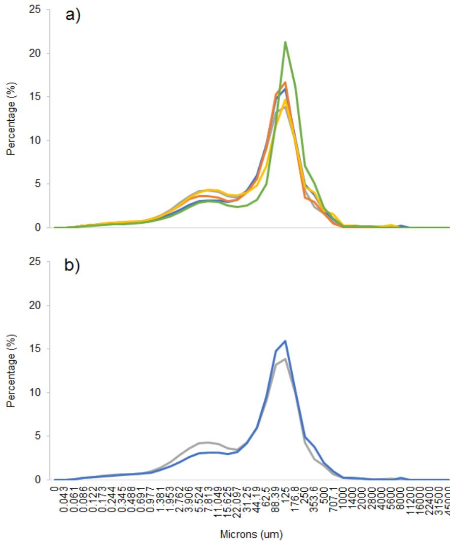
**Figure 8. Particle size distributions for station Re01 within the Coquet to St Mary’s MCZ in 2016 based on: a) 0.095 m<sup>2</sup> Day grab samples (■) and 0.076 m<sup>2</sup> NIOZ corer sample slices (0-5 cm ■, 5-10 cm ■, 10-15 cm ■, and 15-20 cm ■ sediment depth) and b) 0.095 m<sup>2</sup> Day grab samples (■) and 0.076 m<sup>2</sup> NIOZ corer samples for surface sediment only (0-5 cm ■) (© Natural England and Cefas 2022).**
