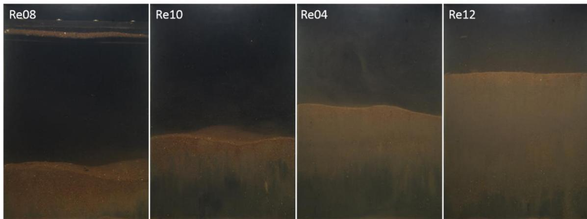
Figure 4. Images collected using the Sediment Profile Imaging (SPI) camera at four stations in the Coquet to St Marys MCZ in 2016. The depth of the apparent redox potential discontinuity (aRPD) layer – where the sediment turns from brown to black – ranges from 4.77 cm to 10.67 cm in these images. © Cefas and Natural England 2016
