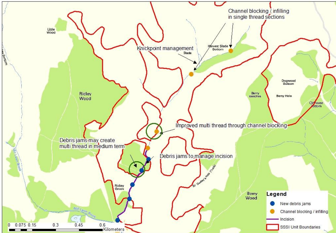
Figure 1-12: Proposed restoration measures for SSSI Unit 126
