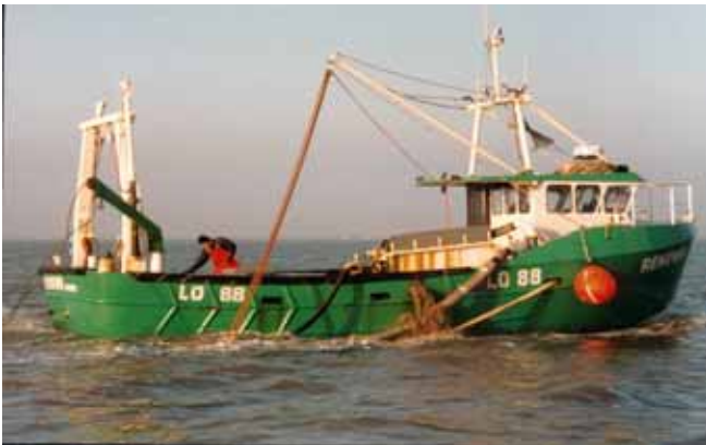
Plate 5 Cockle suction dredging
