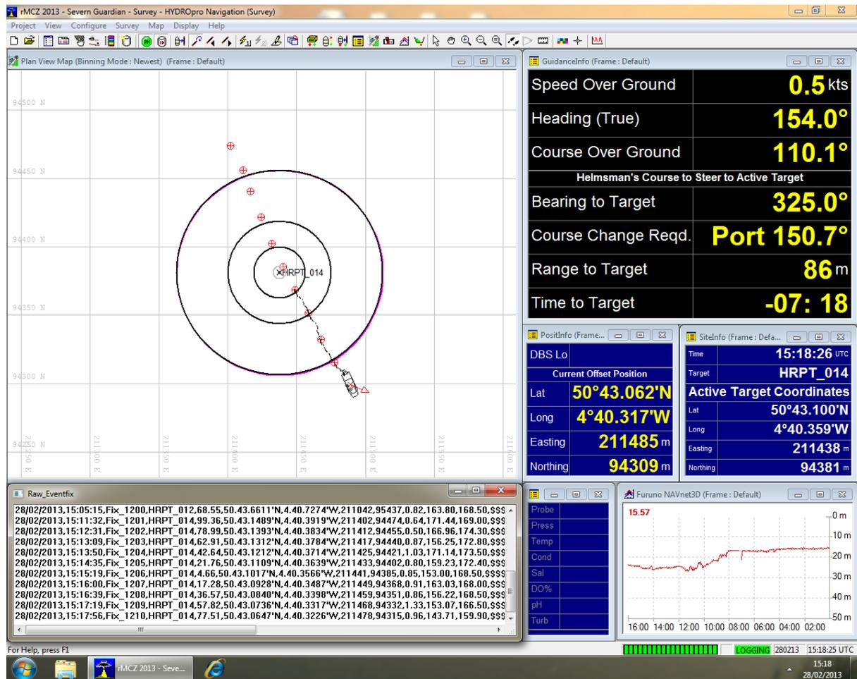
Trimble® HYDROpro™ software screen grab displaying real-time navigation and survey data acquisition (manual fixes).
