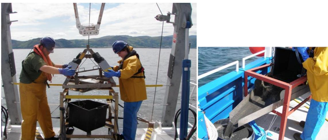
**Figure 4.** Day grab (left) and equipment for sieving benthic fauna samples (right).
