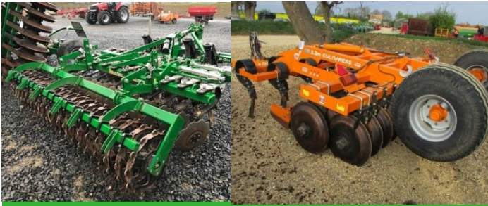
Fig 2: (left) Cultipress and Fig 3: Xpress cultivator machines similar to those used at the Win site
