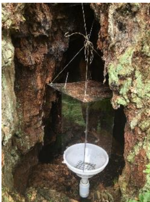
Figure S1.1 Example of a vane trap installed within a hollow in an oak tree. The Perspex panels sit above the funnel which feeds into the collecting bottle. (photo Jon Webb / Natural England)
