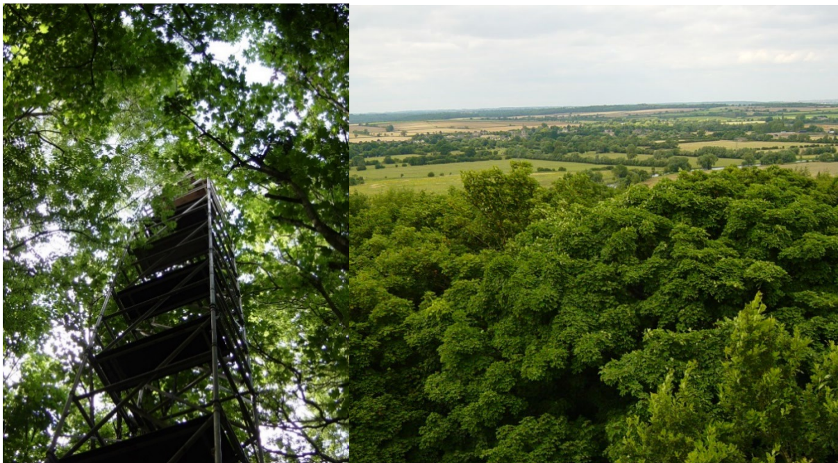
Photos 2.1 and 2.2 Wytham Woods eddy covariance flux tower (left) and view over the canopy from the tower (right) © Natural England / Mike Morecroft
