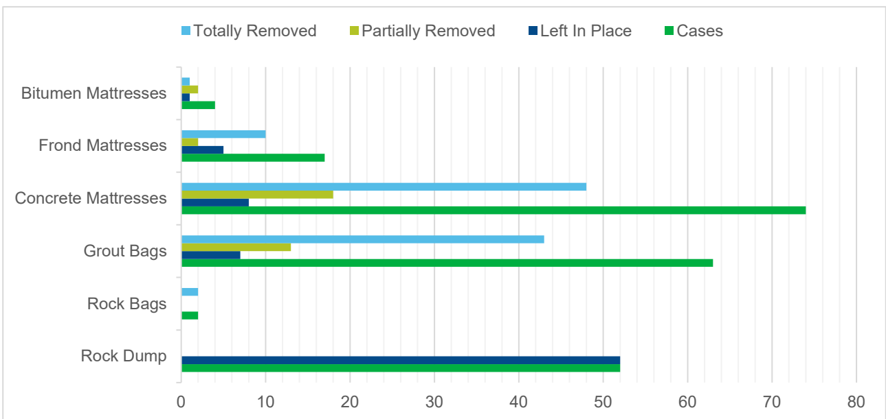
Figure 4-2: Summary of Oil and Gas decommissioning plans
