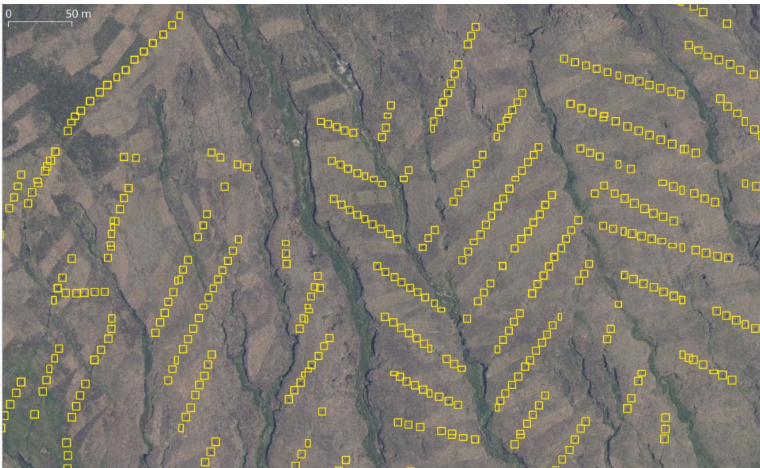
Figure 7-11: Example of dam model output in the North Pennines. Dams detected by the model are shown in yellow. Aerial imagery © 2015 Getmapping plc and Bluesky International Ltd.
