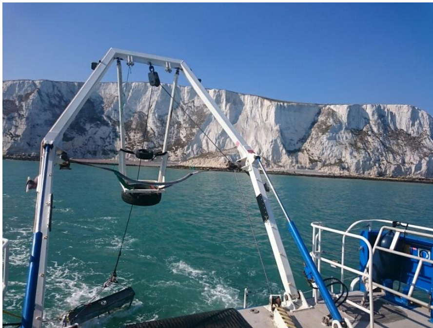
Figure 5. STR SeaSpyder drop camera system being deployed from the stern of the coastal survey vessel.
