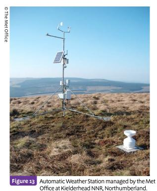
Most of the LTMN sites have an Automatic Weather Station (AWS) which records different meteorological variables. Some sites are already close enough to Met Office weather stations for those data to be representative of the LTMN site.
