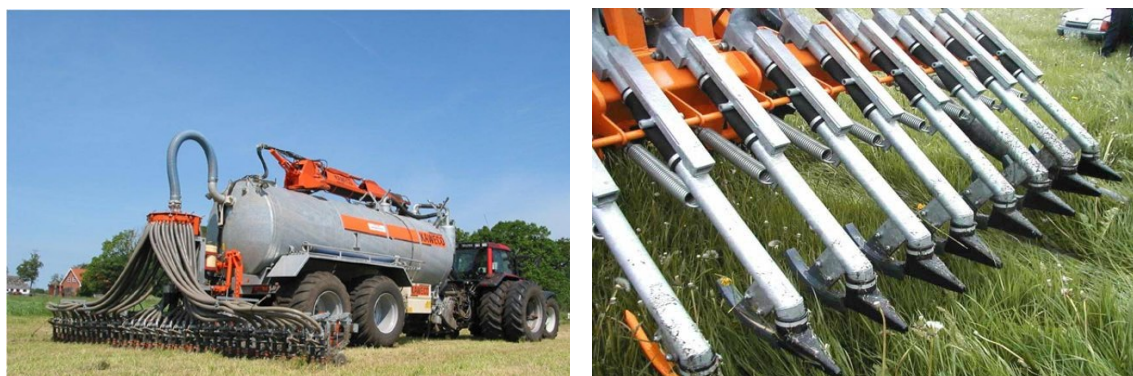
Figure 5. Low emission spreading techniques suitable for grassland: shallow injection (left) and trailing shoe (right)
