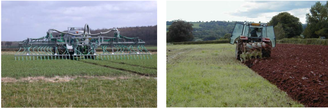
Figure 7. Band spreading of slurry to cereal crops (left) and rapid incorporation of applied manure by plough (right)
