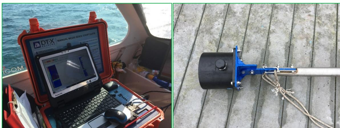
**Figure 4.** The BioSonics DT-X Extreme surface unit (left) and pole-mounted 200 kHz transducer (right).
