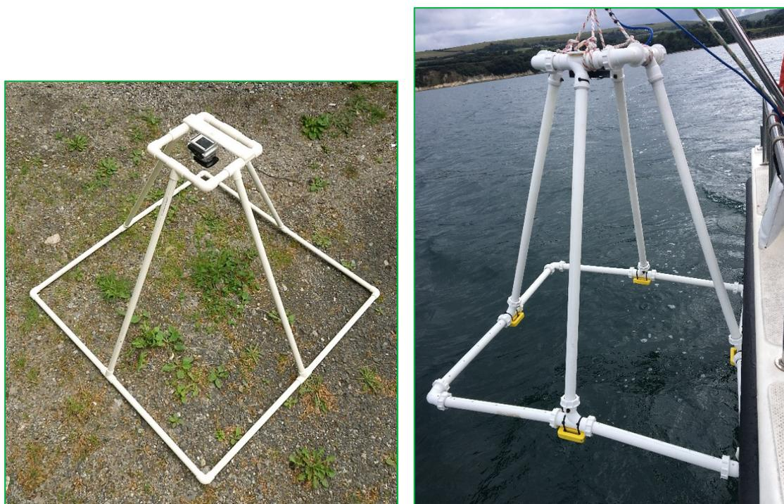
**Figure 3.** The 1 m<sup>2</sup> photo-quadrat with GoPro camera mounted directly above the quadrat.
