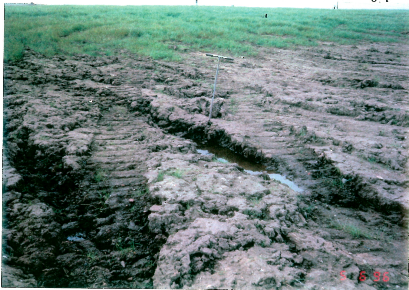
Trafficking of topsoil material.
