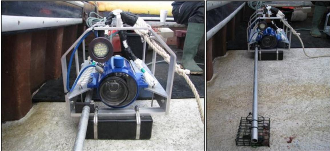
**Figure 2.2** BRUV static frame with bait box developed for the 2011 survey
