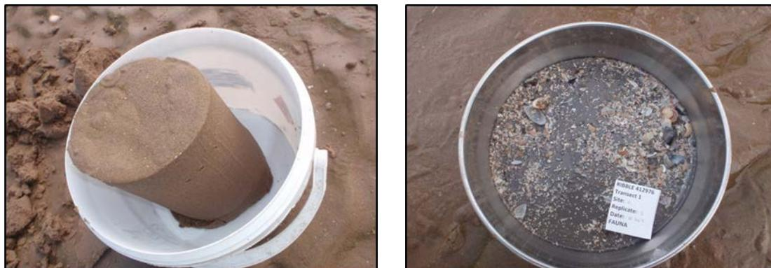
Plate 2. Core sample before (left) and after sieving (right).
