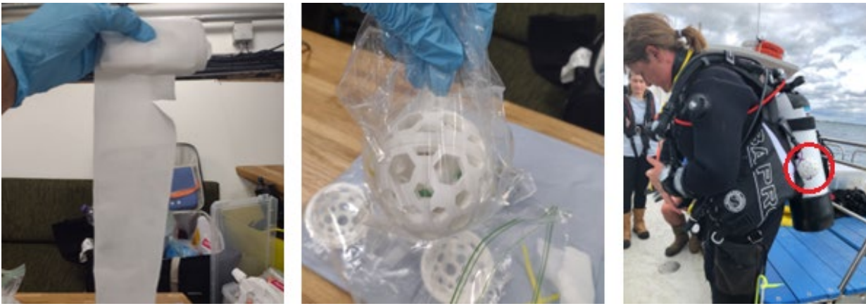
Figure 1. Pictures of metaprobe assembly and attachment to a SCUBA diver. Left: Sterile medical gauze being prepared to place inside a metaprobe. Middle: A prepared metaprobe, ready to cable tie to a diver's equipment. Right: Metaprobe on Natural England diver.
