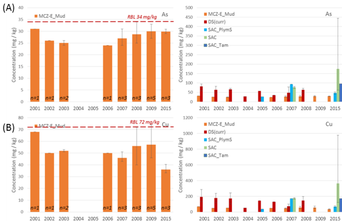
Figure 11. Mean concentration of trace metals considered as primary indicators of presence of dredge material (Okada et al., 2009) during survey years: (A) Arsenic, As; (B) Copper, Cu; (C) Zinc, Zn; (D) Lead, Pb. Metal concentration refers to muddy samples (n) as collected from the deep mud habitat within the MCZ (left panels) and shown in the context of the concentrations in muddy samples from the current disposal site and within Plymouth Sound and Estuaries SAC areas (right panels). Whiskers show range of variation (min and max). Red dashed line indicates regional background levels (RBL).
