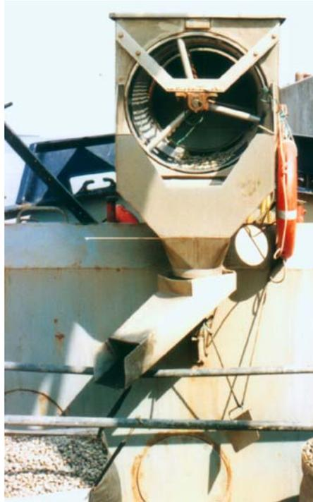
**Figure 2.2** Designs of riddles currently used in the Wash suction dredge fishery for cockles: (a) older style, outboard operated riddle in stowed position (note section nearest camera made of a series of rings, further section made from longitudinal bars); (b) newer style of fixed, fore and aft mounted riddle showing longitudinal bars. Photographs courtesy of ESFJC.
