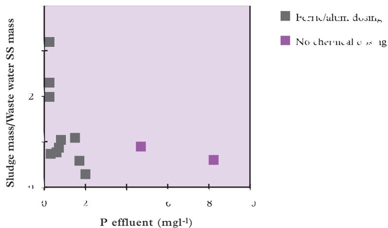
**Figure 8. Relationship between sludge production rate and effluent P concentration (after USEPA 1987)**
